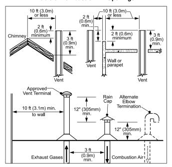
Figure 2. Combustion Air and Vent Through Roof.
